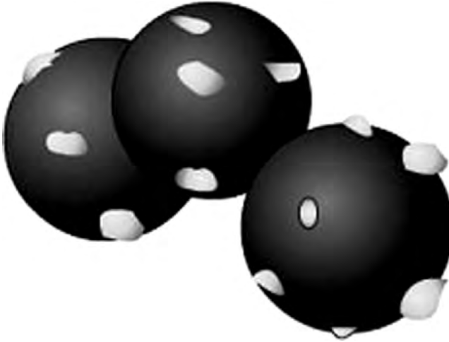
Figure 1-14. Catalyst made of carbon deposited with platinum particles
