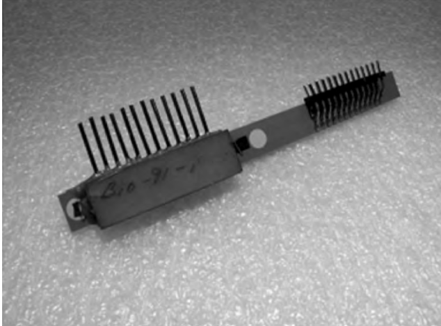
Figure 11-6. A 12-fluid array printhead
