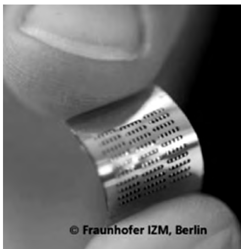
Figure 7-2. Foil type micro fuel cell demonstrator
