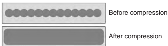
Figure 10-15. Jetted dots used in seal dispensing
