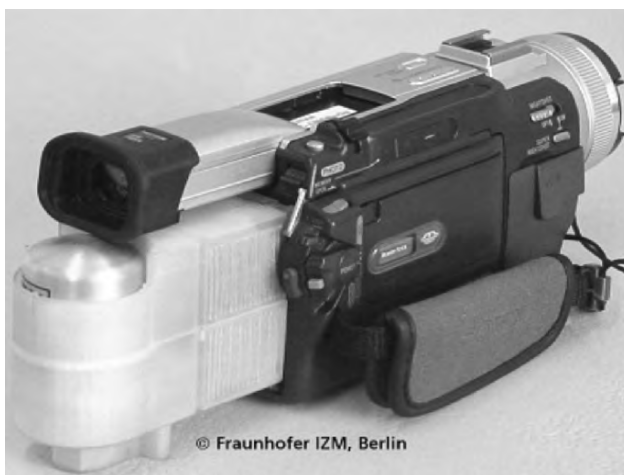
Figure 8-15. PEM fuel cell camcorder demonstration system
