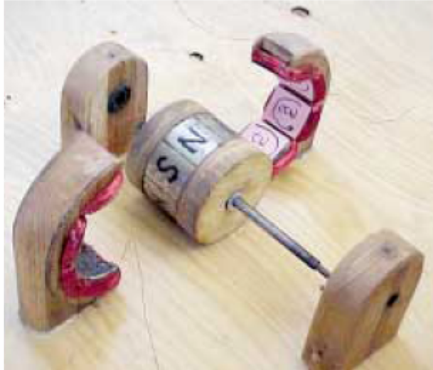
An exploded view shows the armature, stator, and pillow blocks ready to assemble into an alternator.
