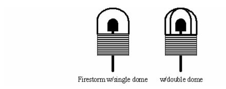
If these plugs ever come onto the market, they have very good potential for plasma fog jet engines as they create a plasma ball type explosion around the electrode. Till then you will have to make your own which could be done by welding a small dome onto the central electrode and then a wire dome over the top. Prototypes may not look that pretty, but they should work.
