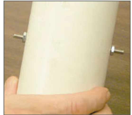
The installed positive electrode connectors
