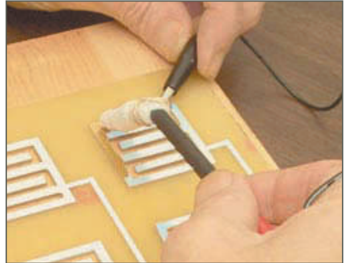
Applying gold plating over nickel plating
