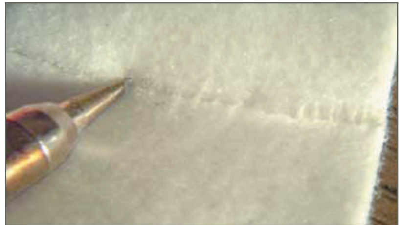
Use a soldering iron to bond the seam of the rolled up felt
