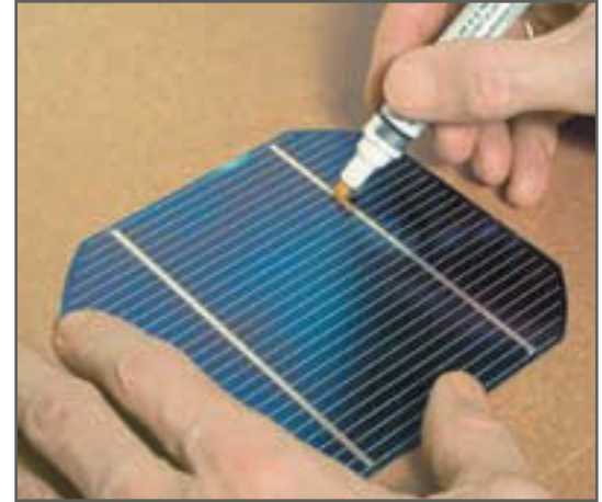
Applying flux to the cell fingers
