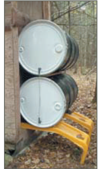
Two recycled 55 gallon drums for short term gas storage
