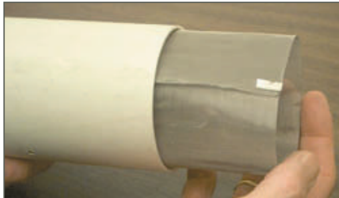
Slip the cylinder back into the pipe
