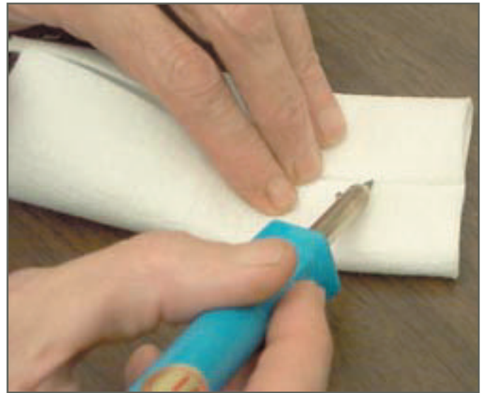
Use a soldering iron to bond the seam of the rolled up felt
