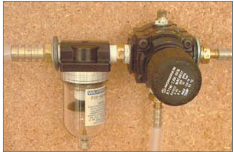
Water filter (left) and regulator (right)
