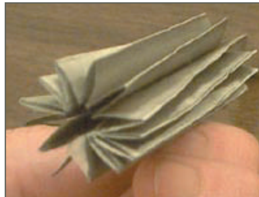
The pleated and rolled negative electrode, ready to install in the bottom cap.
