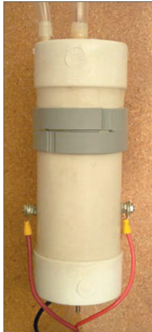
The completed P41 electrolyzer
