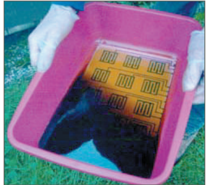
Bathing the plates in etchant solution
