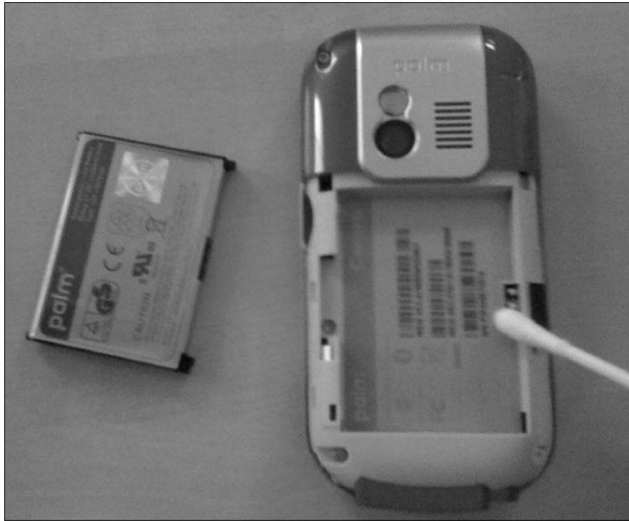
Figure 4-4: Clean your gadget's battery connection to ensure better battery life.
