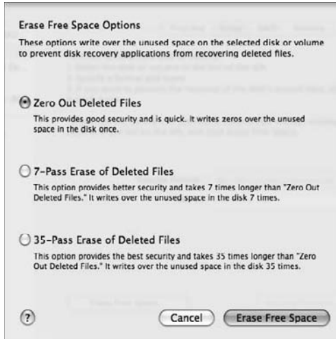
Figure 15-1: The more secure the disk-wiping option, the longer you wait for it to complete.
