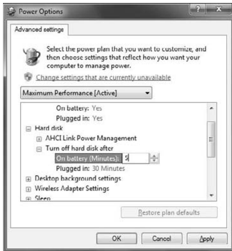
Figure 4-3: Turning off the hard disk to yield big energy gains.
