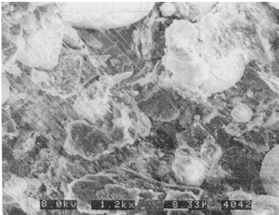
FIGURE 31.2 Scanning electron microphotograph of roll-bonded nickel electrode material. (Courtesy of Evercel Corp.)
