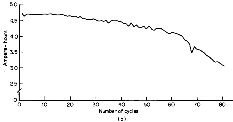
FIGURE 34.20 (a) Discharge characteristics of a \text{Li}/\text{Li}_x\text{NiO}_2 D-size battery. Charge at 0.3 A to 4.1 V. (b) Cycle life characteristics of a \text{Li}/\text{Li}_x\text{NiO}_2 D-size battery. Discharge at 2 A to 2.8 V. Charge at 0.4 A to 4.1 V. Taper to 0.1 mA. (From Ref. 42.)
