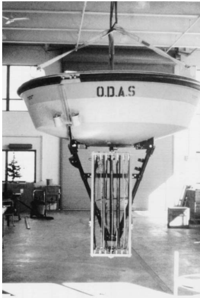
FIGURE 38.31 Aluminum dissolved oxygen flat-plate battery (attached to Woods Hole Oceanographic Institution buoy.) (Courtesy of Alupower, Inc.)
