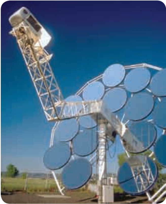
A Stirling engine driven by heat from focused mirrors can produce up to 30 kW of electricity.
