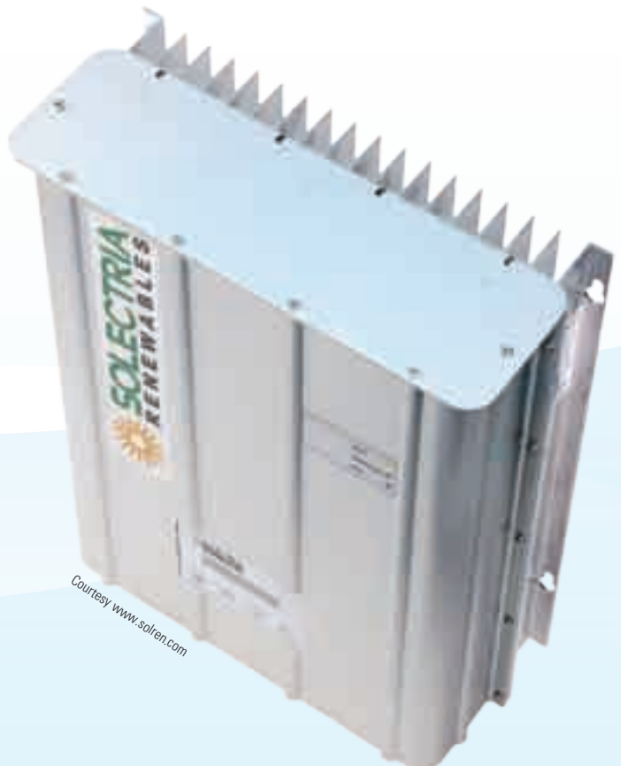
Solectria Renewables PVI 1800 and 2500 series inverters come prewired with DC and AC cabling, and can be integrated with DC and AC disconnect assembly options. The AC output is field-adjustable to 208 and 240 VAC.
