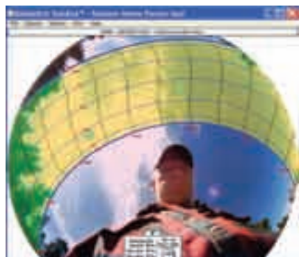
Solar access values can be used to adjust system output expectations.
