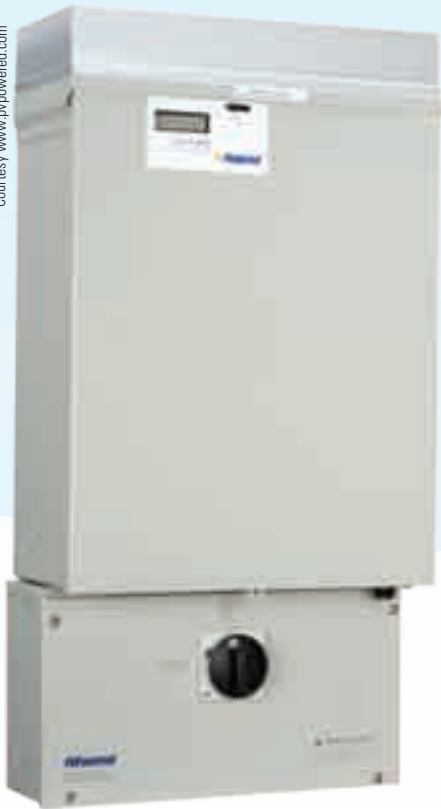
PV Powered PVP series inverters have integrated DC and AC disconnects that meet the UL 98 standard, which means they are considered to be “enclosed and dead-front switches” helpful for installation and inspection.
