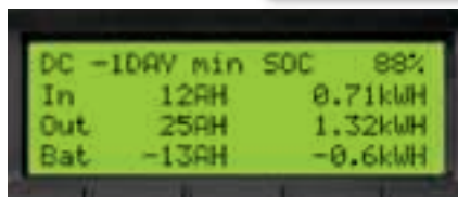
OutBack's FlexNet DC meter allows users to check battery status through a series of displays.
