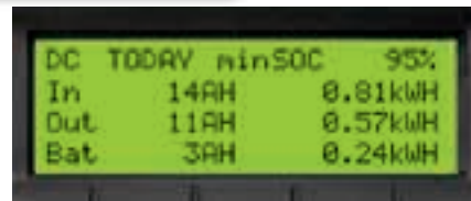
OutBack's FlexNet DC meter allows users to check battery status through a series of displays.
