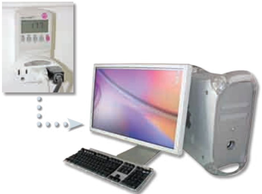
This older desktop computer draws 177 W with an LCD monitor. A CRT monitor could bump power consumption to as high as 300 W.
