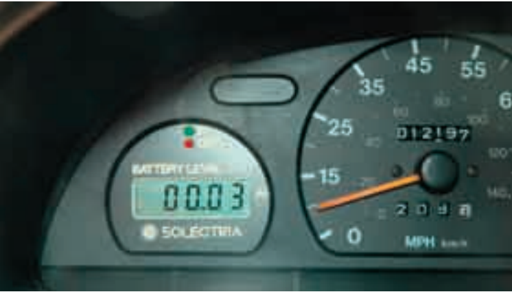
An amp-hour meter is the EV equivalent of a gasoline tank gauge.
