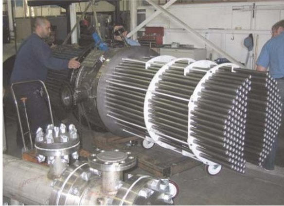
Fig. 9.9 A tantalum metal heat exchanger shown as a concept for scale-up of closed-one-ended all-metal membrane tubes (NORAM) (Courtesy C. Brereton, J. Lockhart, and W. Wolfs, NORAM)
