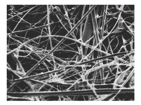
Figure 2.16 The surface of a fibrous filter.
