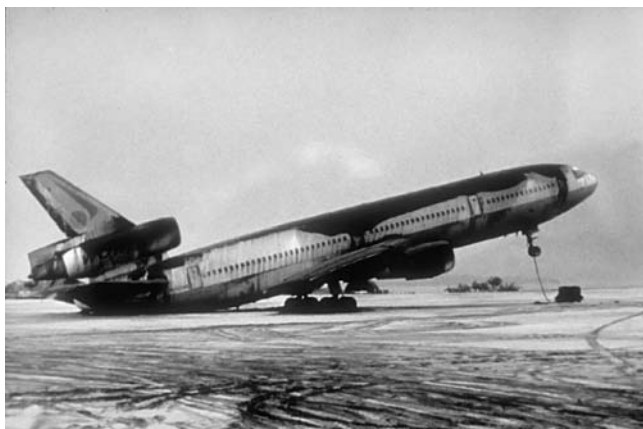
A World Airways DC-10 jet at Cubi Point Naval Air Station is covered with volcanic ash after the eruption of Mount Pinatubo, Philippines, June 17, 1991. Ash is very abrasive and can cause engines to stall or fail if an airplane flies through an eruption cloud. The eruption of Mount Pinatubo caused 11 commercial aircraft emergencies. (Courtesy of the USGS)
