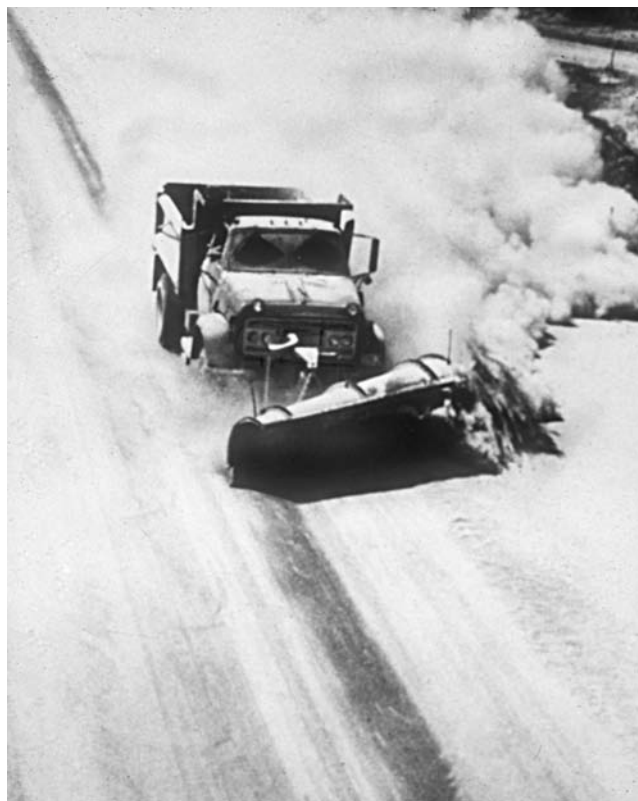
This regular snowplow is plowing the road on May 18, 1980, in Washington. However, it is not plowing snow, it is plowing volcanic ash from the eruption from Mount Saint Helens. Ash blanketed the area around the volcano so deeply that it looked like there had been a gray snowstorm. The problem is that ash is much heavier than snow and thus caused many roofs to cave. (Courtesy of the USGS)
