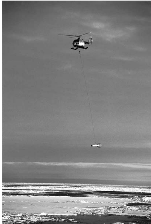
Fig. 3.8 Photograph of Alfred Wegener Institute's fully digital helicopter electromagnetic (HEM) bird in operation in the Arctic.
