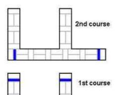
Garden walls built using Flemish bond are one bricks wide. As with any wall built of brick, no two adjacent vertical joints should be in line.
