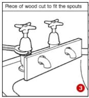
You can cut a notch in a piece of wood and use it as a lever to hold the taps steady. Alternatively, mark two holes where the spouts are positioned and drill two holes so the piece of wood can be slipped over both spouts to hold the taps steady (3).
