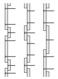
Board and batten siding can have a variety of appearances depending on the width of boards and battens. A reverse board and batten pattern is achieved by placing wide boards over the narrow battens.
