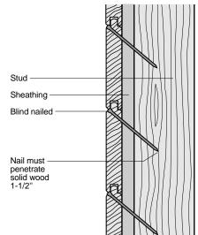
For 4-and 6-inch widths of tongue and groove siding over solid wood sheathing, blind nailing is possible using one 8-penny finishing nail per bearing.
