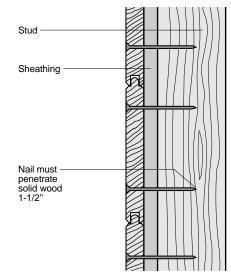
Tongue and groove siding 8 inches or wider should be face-nailed, using two 8-penny nails per bearing.
