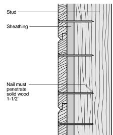
For 6-inch V Shiplap patterns, use one nail per bearing with the nailing point one inch from the overlapping edge. For patterns 8 inches and wider, face nail with two siding nails per bearing. Position nails one quarter the width of the material in from each edge.
