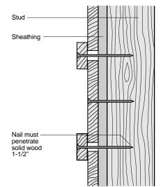
Space underboards at least 1/2 inch apart and nail with one nail per bearing through the center of the material. For boards wider than 8", use two face nails evenly spaced. Wider spacing may be used with wider battens. Nail batten strips through the center so the nail shank passes through the space. Make certain the batten laps the underboard at least 1/2 inch on both sides.
