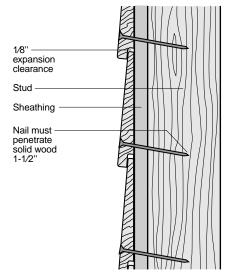
Face nail with one nail only per bearing. Position material to allow expansion clearance of 1/8 inch. Drive nail about one inch above lower edge of course.
