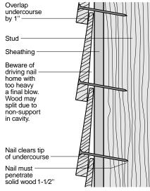
Face nail with one nail only per bearing. Drive nail so shank just clears the tip of the preceding undercourse. The space between the nail shank and the tip of the preceding course should not exceed 1/8 inch.
