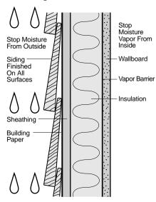
Proper interior and exterior wall construction prevents moisture problems. Building paper should have a permeability rating of 5 perms, the vapor barrier, a maximum of 1 perm.
