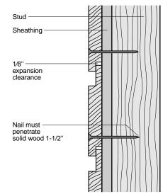
Use one nail an inch from the lap for 6-inch Channel Shiplap. Face nail with two nails per bearing for 8-inch and wider patterns. Space nails 1-1/2 inches from edge of overlap and two inches from edge of underlap for 8-inch boards. Nail wider patterns proportionately.
