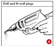
Remove the assembly, then drill and plug the wall-fixing holes (4). Also drill a hole for the 21mm (3/4in) overflow pipe, allowing for a fall to the outside.
