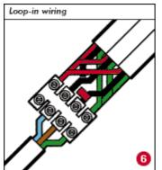
(6). Start by connecting all the cable earth cores to connector 1, the black core of the switch cable to connector 2, the other black cores to connector 3 and all the red cores to connector 4. Connect in the flex next, taking the earth core to connector 1, the brown to connector 2 and the blue to connector 3.
