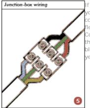
If only one cable is present, you need three strip connectors to link it to the flex tail from the light fitting. Connect the red cable core to the brown flex core, black to blue and earth (green-andyellow) to earth (5).
