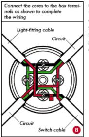
Connect the cores to the box terminals as shown to complete the wiring (8), screw the box to a joist and fit its cover. Restore the power and test the operation of the light.
