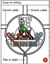
Modern ceiling roses have a bank of terminals on their baseplates, and there will be at least two and probably three cables present (1). The circuit cable loops into and out of each rose in turn, terminating at the last rose of the circuit. A switch cable is wired into each rose and runs down to the switch that controls it. This is known as loop-in wiring.
