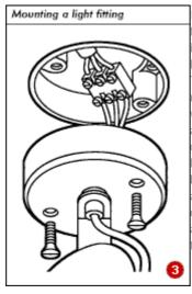
If the new light fitting has a flex tail, you have to use insulated strip connectors to link this to the circuit wiring. The connection must be made inside an enclosure which is formed by recessing a round conduit box into the ceiling and then mounting the light fitting immediately below it (3). You will need access to the ceiling void to do this - easy if there is a loft above, but involving lifting floorboards otherwise.
