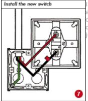
Install the new light fitting and its switch (7). Then run a cable back from each component to the new junction box.
