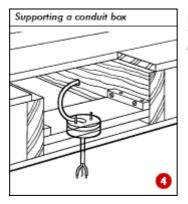
Feed the cable(s) down through the hole and into the conduit box (4).
