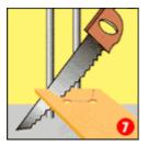
If you need to fit your flooring around pipes, start by measuring the diameter of the pipe then drill a hole, 20mm larger than the pipe diameter, in the laminate board. Saw a section out of the board which goes through the hole (7) so that it can be laid around the pipe and replace the sawn out section and glue in to place.
