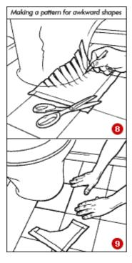
Awkward shapes around sink pedestals, door architraves etc, are best overcome by first making a cardboard pattern of the precise shape and transferring this to the tile (8 & 9).
