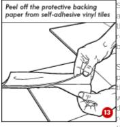
Self-adhesive vinyl tiles have a paper backing to protect the adhesive (13). Do not remove this until the tile is to be laid.
