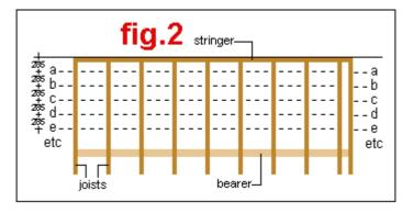
Step (3) Lay and nail every third row of decking board on the building side of the <u>chalklines</u>.
