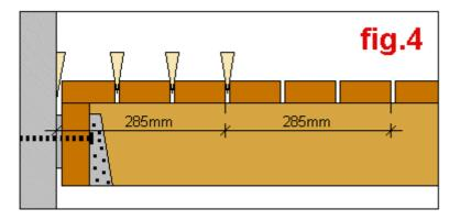
Step (5) Cut the joist ends vertical and flush with the outside edge of the last decking board. Nail the boundary joist around the perimeter of the deck making sure the top of the boundary joist is is flush with the top of the decking. See diagram below.
