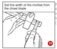
When adjusting the gauge to the width of the mortise you need, set the points directly from the width of your chisel (12).
