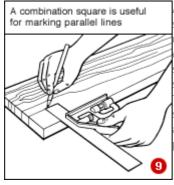
A combination square has several uses. Most can be used as either internal or external try squares, mitre squares, depth gauges, straightedges and steel rules. They are usually fitted with a small spirit level. They are also very useful for marking parallel lines (9).
