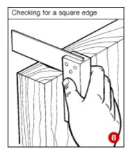
The try square is also used to check that faces are at 90 degrees to each other. The stock of the square is laid flat against one face of the work and a check is made visually to see if light appears under the steel edge (8). If it does, more planing is necessary on the opposite side to the light, to square up the work. The try square is also used to check internal and external angles of assemblies.
