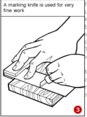
For very fine work to be cut, use a marking knife or a craft knife. These not only mark but sever the fibres very slightly to enable further cutting to be very exact (3). The severed fibres leave a whisker-free cut edge.
