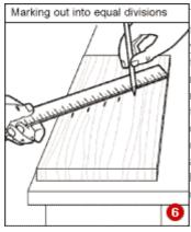
The simplest way to divide the work equally is to hold your rule diagonally across the surface and decide how many divisions you want to make. Be sure that the end of the rule is level with the edge of the material and the divisions will fall equal automatically. This is very handy for marking out dovetails and other joints (6).
