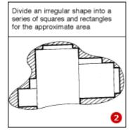
The area of a large, irregular shape can be approximated by measuring square or rectangular areas within it and adding the measurements of these areas together. Make an allowance for the small, irregular areas left at the edges (2).
