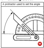
The sliding bevel is a specialised type of square, which is infinitely adjustable and which is used for marking and transferring pre-set angles. This is useful for setting out angles for corner cupboards, steps, dovetails and multi-sided picture frames. It is usually set either from an existing angle or by using a protractor (10).
