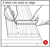
Using a rigid rule held on edge, with your fingers against the edge of the material being cut, is a quick way to step off the width (5).
