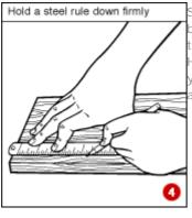
Steel rules are very useful, but they do have a tendency to slip on smooth surfaces. Hold the rule down well, with your fingers spread wide along the rule (4).
