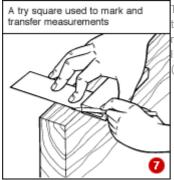
The most basic square is the try square. Use a pencil or marking knife to mark your line against the steel edge
