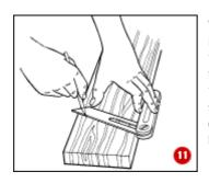
When using the sliding bevel it is essential to ensure that the stock of the tool is held firmly against the edge throughout (11). Tighten sliding bevels well, and occasionally check that they haven't moved in use.
