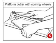
Alternatively, use a tilesnapping tool with the jaws directly aligned with the score mark or use a platform cutting table with a scoring wheel to score and snap the tiles.
