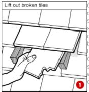
On pitched roofs the job of detection should be easier since you can identify slipped slates and tiles from the outside. Remove and replace broken tiles by carefully lifting them clear of the nibs on which they rest. It can sometime help to insert wooden wedges under the overlapping tiles first (1).
