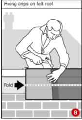
Gently tread the felt down as you pull off the paper. When the first half is stuck down, repeat for the second half, then stick down the drip edge pieces. These will run over the edge of the roof and into the gutter. They should be nailed face down and then folded upwards to form a double thickness drip over a wooden batten (8). If you aren't sure how this is done, look at a few flat roofs in your area.
