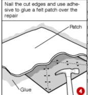
Tack the flaps with galvanized felt nails, otherwise known as clout nails. When this layer has dried, apply more adhesive and stick a patch of felt over the top so it overlaps the repair by 150mm (6in) on all sides (4). To help it stick down, place some slabs on it for a few days.
