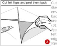
Cut back the felt with four diagonal lines to create envelope flaps. Gently peel back the felt and expose the underlayer of roof decking
