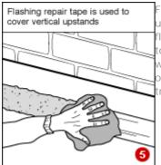
Flashing and joins to vertical upstands can be covered by flashing repair tape. Be sure to apply enough pressure when pressing it in place in order to get rid of any trapped air underneath (5).
