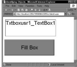
Figure 5-7: Identifying object names as they appear on the client-side.
