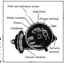
Figure 12-15: The anatomy of a nonelectronic distributor.
