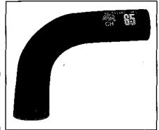
Figure 14-5: A preformed radiator hose.
