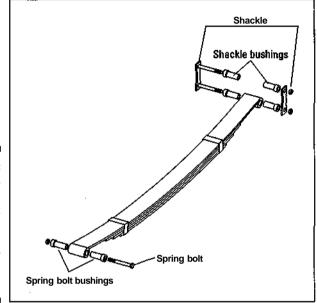
Figure 11-8: Leaf springs bend but do not break because they can slide flexibly on one another.
