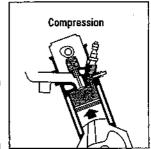
**Figure 7-8:** Compression stroke.
