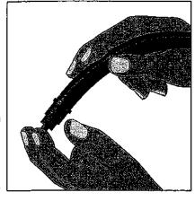
Figure 13-8: One way to checkyour PCV valve.
