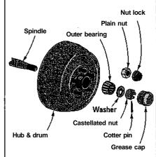
Figure 18-4: The things you have to remove to get at your drum brakes.
