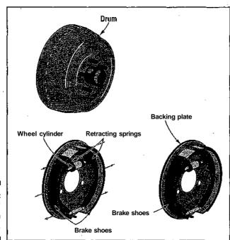
Figure 18-6: Anatomy of a drum brake.
