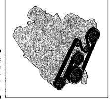
Figure 3-3: Serpentine multiaccessory drive belt.
