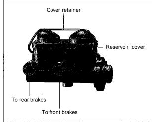
Figure 10-3: A metal master cylinder.
