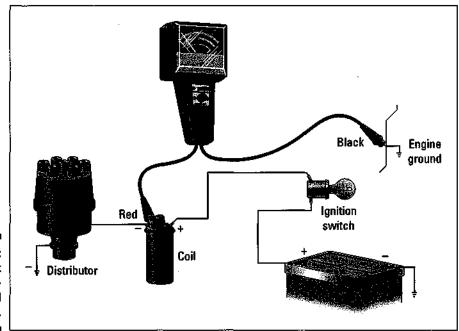
Figure 12-42: How to hook up a twoclip dwell meter.
