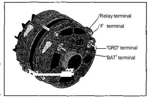
Figure 5-6: The alternator.
