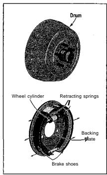
Figure 10-5: Anatomy of a drum brake.
