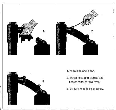
Figure 14-9: How to install a hose.
