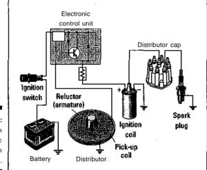
Figure 5-9: electronic ignition system.
