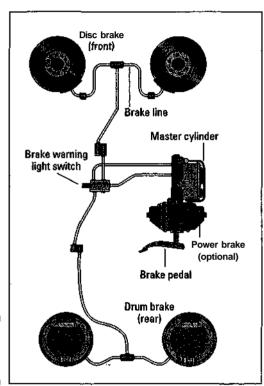
Figure 4-12: The brake system.
