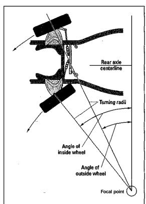
Figure 19-7: Turning radius.
