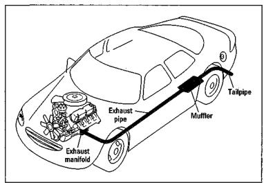
Figure 4-11: The exhaust system.
