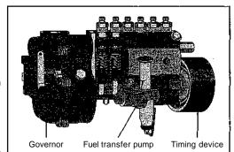
Figure 7-5: Fuel injection pump.
