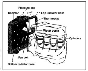
Figure 8-1: The cooling system.
