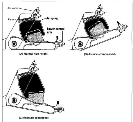
Figure 16-10: How air springs work.
