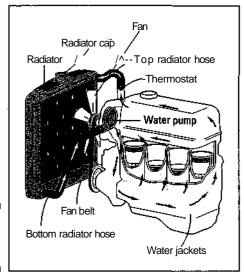
Figure 4-9: The cooling system.
