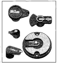
Figure 5-14: Types of rotors.
