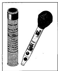
Figure 3-7: Battery tester.
