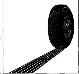
Figure 19-9: It's time for new tires when tread-wear indicators appear.
