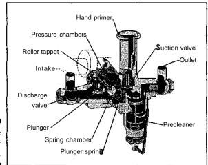
Figure 7-6: Fuel transfer pump.
