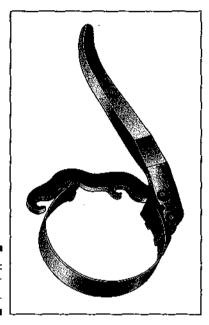
Figure 15-5: An oil filter wrench.
