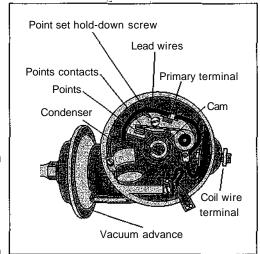
Figure 5-15: Inside a nonelectronic distributor.
