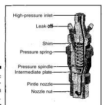
Figure 7-4: Anatomy of a fuel injector.
