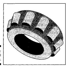
Figure 18-11: Awheel bearing.
