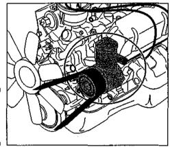
Figure 3-14: The powersteering pump.
