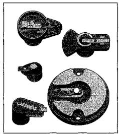
Figure 12-16: Various types of rotors.
