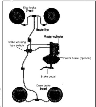
Figure 10-1: The brake system.
