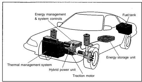
Figure 7-12: A hybrid engine.
