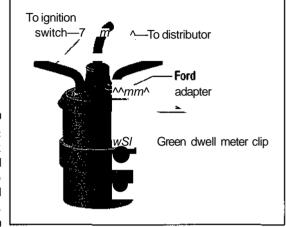
Figure 12-44: How to hook up a dwell meter to some Ford cars.
