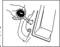
Figure 13-19: Checking compression.
