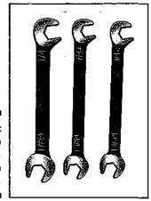
Figure 2-6: Use ignition wrenches for ignition work.
