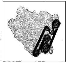
Figure 14-10: Serpentine multiaccessory drive belt.
