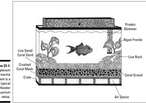
Figure 23-1: A plenum marine system is a typical saltwater aguarium
