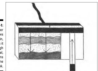
Figure 6-1: A power filter draws water in, passes it through charcoal, and returns it to the tank.
