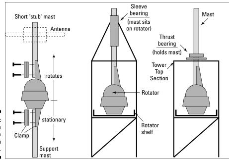
Figure 12-5: Mounting a rotator on a mast and on a tower.
