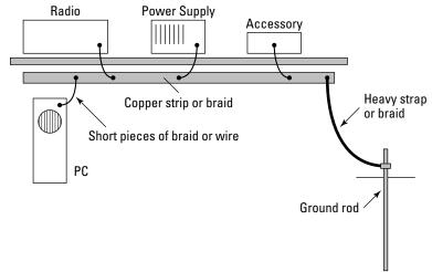
Figure 13-9: Create grounding for RF signals.
