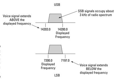
Figure 8-2: The Upper Sideband and Lower Sideband frequencies.
