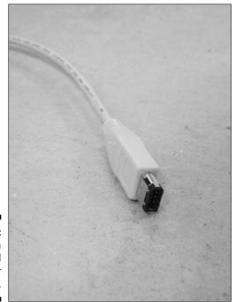
Figure 5-10: FireWire is a high-speed data transfer protocol.
