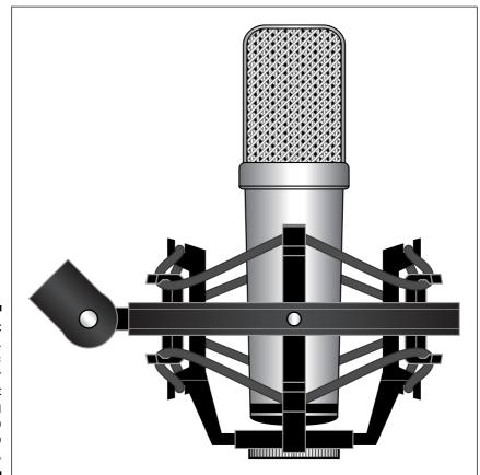
Figure 1-2: A mic. Use a mic when your instrument can't plug directly into your audio interface.
