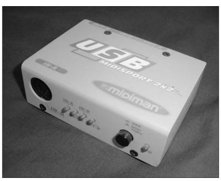
Figure 4-11: A MIDI interface is necessary if you want to connect your instrument to a computer.
