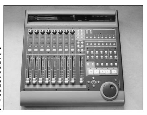
Figure 1-6: A computercontrol surface offers you real knobs and faders and still uses the mixer that's part of your software.
