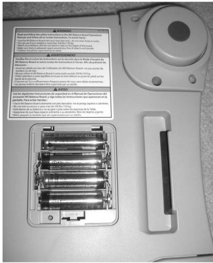
Figure 13-1: The Balance Board battery housing and SYNC button.
