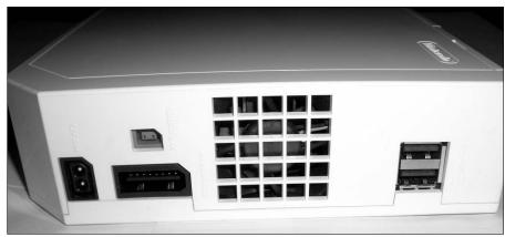
Figure 2-3: The Wii's rear connections.
