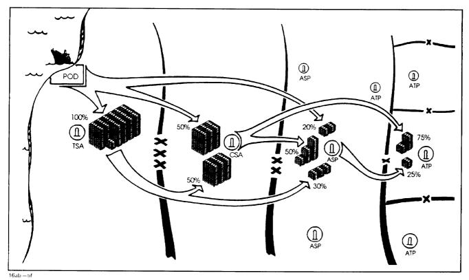
Figure 1-9. Flow of ammunition within the theater utilizing MOADS.
