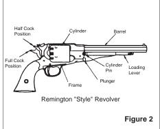
7. During reassembly, LIGHTLY oil all moving parts and grease the grooves of the cylinder pin.
