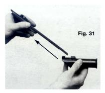
The trigger group may be removed from the receiver for further cleaning of the receiver and trigger group. It is recommended that a thorough cleaning be performed every 300 rounds.
