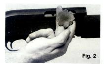
The bolt handle of your shotgun is protected from damage by a rubber pad. Simply slide your fingers under the rubber pad as shown in Fig. 2 and lift the pad completely off the bolt handle.
