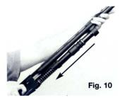
Continue pulling the bolt handle back while inserting the barrel until the bolt is in its rear locked position and the barrel is completely seated in the receiver. The barrel should mate to the receiver at this point in the assembly as shown in Fig. 11.
