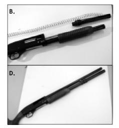
Magazine Tube Extension: Increases the Magazine tube capacity to hold 4 rds of 3.5" 12ga
