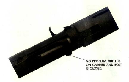
If you see that a shell has slipped out of the magazine, under the closed bolt resting on the shell carrier, THIS IS NOT A JAM. Simply fire the gun or cycle the action by hand and the SPAS 12 will feed that shell into the chamber without allowing another shell to come out of the magazine. You need not use the magazine cut-off button or do anything else. The next shell will feed normally.
