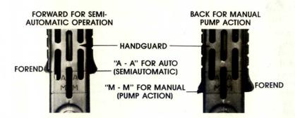
To switch from semiautomatic mode to pump mode, push in the selector button and slide the forend back so the rear of the forend lines up with the "M - M" line on TOP of the handguard.
