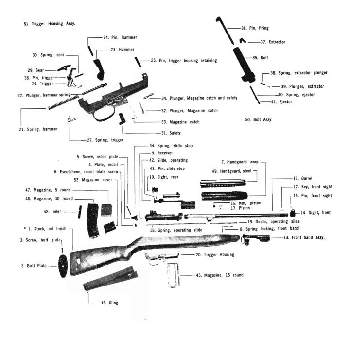
**CAUTION:** This is a gas operated weapon, and is manufactured to rigid specifications. To insure proper functioning the weapon should be used with ammunition made to proper specifications. This will insure satisfactory feed, functioning and safe operation. Malfunctions are usually attributed to (1) improper ammunition (2) damaged magazine (3) magazine not inserted properly. Front sight is adjusted by flat filing center post to bring group up to desired location.
