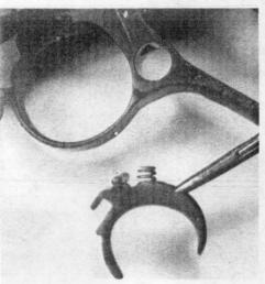
18. The trigger may easily be moved to the left and taken out of the frame, along with its attached spring.
