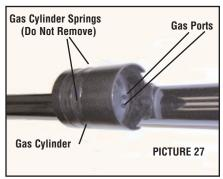
13. Spray Rem™ Action Cleaner in the gas cylinder. Push a wire brush the size of the gas cylinder through the gas cylinder several times and wipe dry. DO NOT REMOVE THE GAS CYLINDER SEAL OR GAS CYLINDER SPRINGS. See Picture 27 and 28.
