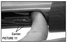
Push up to four (4) shells of the correct gauge and length one at a time fully forward into the magazine tube. Make sure the rim of each shell engages the feed latch and is held inside the magazine tube.
