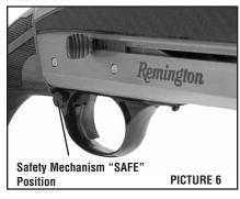
Always engage the safety mechanism by moving the safety button to the shooter's right before handling, loading or unloading the firearm.
