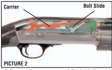
bolt assembly moves rearward, it extracts the spent shell from the chamber and recocks the hammer. The rate controller (not shown) regulates the speed of the bolt. Once the bolt is fully open, the carrier sweeps downward (Picture 3) ejecting the spent shell out the ejection/loading port (Picture 4).
