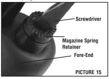
Push down on the screwdriver and magazine spring retainer approximately one (1) inch or until you can turn the screw driver.
