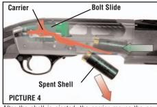
After the shell is ejected, the carrier moves the new shell released from the magazine (Picture 5) and places it in front of the bolt. Completing the cycle, the bolt moves forward chambering the new shell. See Picture 2. Once the last shell has been discharged, the bolt assembly locks in the open position.
