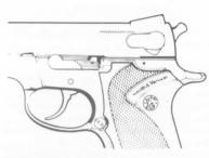
(Figure 4) Fire Position - Left Side Safety
