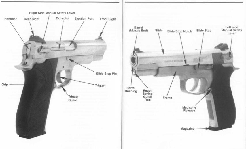
Note; Parts for a magazine release for left-handed shooters are available for 10mm pistols only.
