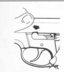
(Figure 7) Field Stripping Aligning Stop Notch & Slide Stop
