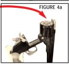
Push back the barrel latch and rotate the barrel downward. With the barrel pointed in a safe direction, continue to open the frame and barrel until the extractor completes its cycle and snaps back into the cylinder. (Figures 4 & 4a)
