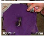
I use a very strong cleaner on the exterior and interior of the bolt. Break Free Powder Blast is a good cleaner for this. It is non oil based and really removes crud without having to scrub and without leaving any residue.
