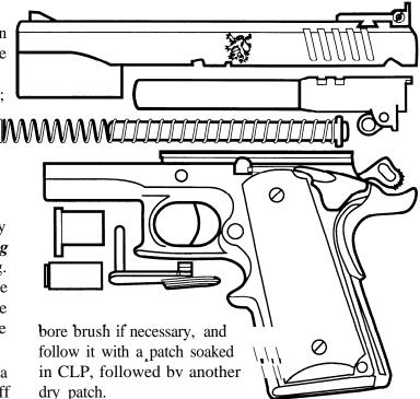
With a quality lubricant designed for stainless steel (such as FP-10, Energy Release, etc.), put a few drops on the running, or friction surfaces in the slide i.e., where the barrel rides, the slide rail surfaces where they match the frame, and on the disconnector ramp. These areas usually show wear and shiny patches. NEVER squirt oil into the frame.
