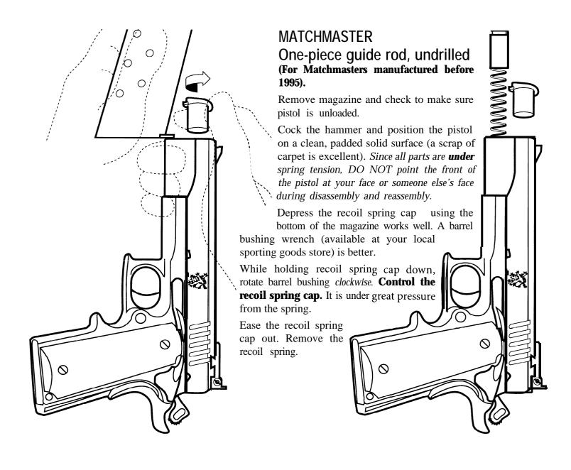
Move slide back until take-down notch is above slide stop tab.
