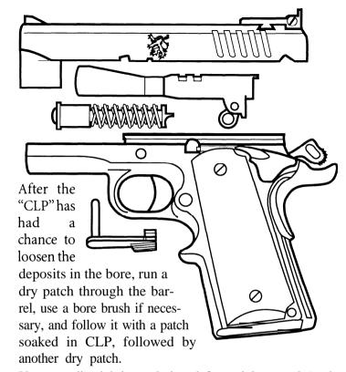
Use a quality lubricant designed for stainless steel (such as FP-10, Energy Release, etc.). Put a few drops on the running, or friction surfaces *in the slide only;* i.e., where the barrel rides, the slide rail surfaces where they match the frame, and on the disconnector ramp. These areas usually show wear and shiny patches. NEVER squirt oil into the frame. Do not over-oil. It can be detrimental to the proper function of the pistol.
