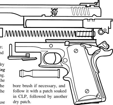
With a quality lubricant designed for stainless steel (such as FP-10, Energy Release, etc.), put a few drops on the running, or friction, surfaces *in the slide only;* i.e., where the barrel rides, the slide rail surfaces where they match the frame and on the disconnector ramp. These areas usually show wear and shiny patches. *NEVER* squirt oil into the frame.
