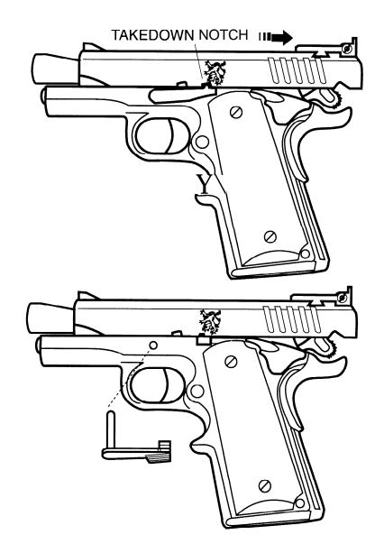
Remove slide unit by moving it forward and off the frame.
