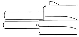
move the slide back until the slide stop engages. Look at the guide rod. If there is a tiny hole drilled through it, you have a captive system (page 15). If there isn't, you have the undrilled system (page 26).
