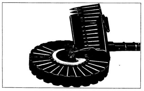
PLATE VIII-LOADING TOOL WITH MAGAZINE IN POSITION
