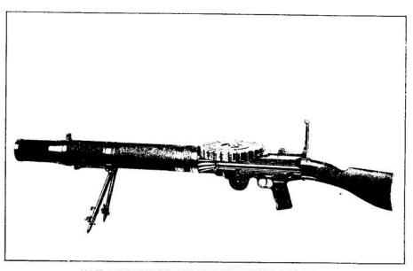
PLATE I-GUS COMPLETE WITH MAGAZINE AND BIPOD FIELD MOUNT
