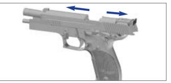
6. Now slip complete assembly (slide 50, barrel 57, recoil spring 62 and recoil spring guide 61) forward and off the frame.
