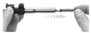
CAUTION: The firing pin is under spring tension when installed in the bolt head. Use caution during removal to prevent injury to yourself and others. The use of eye protection is recommended.
