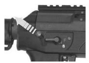
4. Remove the pivot pin (forward pin): unscrew the pivot pin screw (left side) and remove the pivot pin from the trigger casing;
