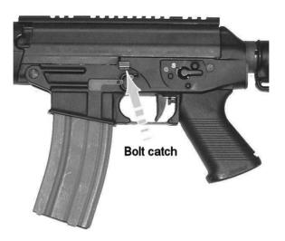
CAUTION: Dropping or jarring the rifle with the bolt locked open can cause the bolt catch lever to disengage. If a magazine, loaded with ammunition, is inserted in the rifle when this occurs, a round will chamber with the potential for an unintentional discharge. ALWAYS handle the rifle as if loaded whenever a magazine is inserted in the rifle. ALWAYS place the safety lever in the "S" (SAFE) position and unload the rifle whenever shooting is complete.
