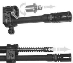
12. Push the operating rod assembly forward and remove from the gas tube;
