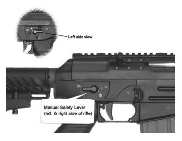
**The safety is "on"** when the safety lever is in the "S" (SAFE) position and the trigger guard is closed. In this position, the rifle cannot be fired with a normal pull of the trigger.
