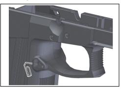
Fig. 7, Releasing the magazine catch stop (illustration without trigger)
