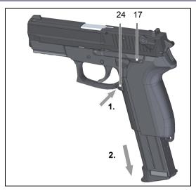
Fig. 4, Removing the magazine
