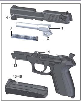
Fig. 18, weapon stripped for cleaning
