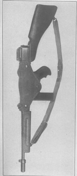
for the protection of gun mechanism—can be instantly taken off by one continuous After being detached in an emergency, a leather thong holds cover on gun so it will not be lost. Thompson Gun breech cover for the pull on cover flap. After b
