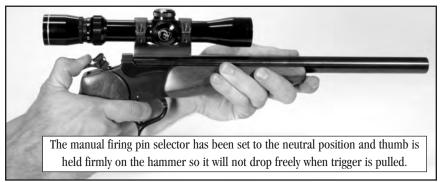
4. Carefully lower the hammer forward, allowing the automatic hammer block to engage in the "at rest" position as shown on the next page.
