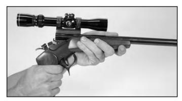
Pulling back on the trigger guard spur will allow the barrel to pivot downward. To close the G2 Contender, pull the barrel upward while securely holding the grip of the G2 Contender stationary with your right hand. Practice opening and closing the G2 Contender pistol or rifle before attempting to load and fire this gun.
