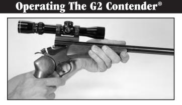
The G2 Contender is a single shot, break-open style firearm. To open the G2 Contender, hold the gun with your left hand at the balance point on the forend. (Use right hand if you are left handed). With your other hand, pull rearward and upward on the trigger guard spur with your trigger finger. Place your finger low on the spur for maximum leverage, and give it a fast, sharp pull. Pull rearward and up at the same time.
