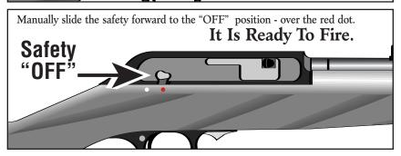
The Model R55 safety can only be engaged in the rearward "ON" position when the hammer is cocked. You will be unable to engage the safety in the rearward "ON" position when the hammer is in the uncocked position.
