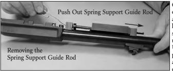
6. Put on a pair of safety glasses as you will now be removing a spring which is under tension. Using a 1/16" punch, nail, or a large straightened paper clip,
