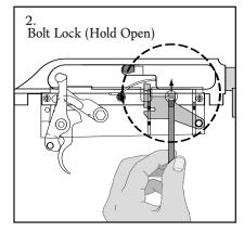
2. Insert a pencil (or wood dowel) into the magazine well and press up on the
