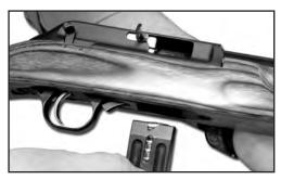
The bolt of your Model R55 can be in 2 positions. It can be locked in the rearward position, held by the bolt stop, or it can be fully forward against the chamber of the barrel.
