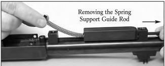
port guide rod towards the muzzle with your other hand until the spring is free from the rod. It is still under tension; do not let it go. Pull the spring out of the
