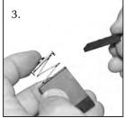
4. Thoroughly clean the inside of the magazine and lightly lubricate it. Wipe the spring off and lightly lubricate it as well.
