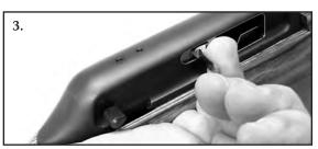
3. Pull back on the bolt handle. (with an empty magazine inserted, the bolt will remain locked in the rearward position)
