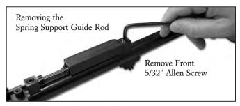
5. To remove the spring support guide rod from the barrel/receiver assembly, back out (or remove completely) the spring guide rod locking screws with a 5/32" Allen wrench.
