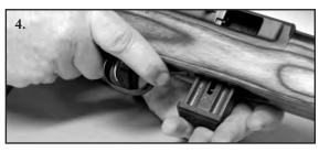
4. Press the magazine release located at the front of the trigger guard, making sure that one of your hands is under the magazine to catch it and stop it from falling to the ground. (preventing any damage to the magazine).
