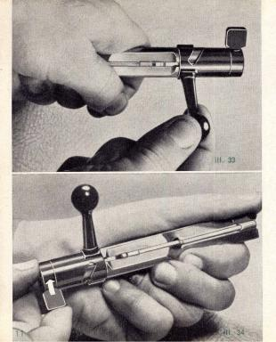
**JII. 33.** The bolt is uncocked. Note the position of the bolt handle. The inner end of the bolt handle now stands close to the striker groove in the bolt.
