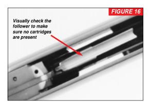
IMPORTANT: ALWAYS VISUALLY NOTE, BY LOOKING THROUGH THE TOP OF THE OPEN RECEIVER, THAT THE MAGAZINE FOLLOWER IS SHOWING—AND NOT A CARTRIDGE (SEE FIGURE 16).
