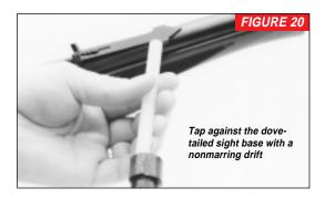
sight base (where fastened to the barrel) to the right, your gun will shoot more to the right. An adjustment to the left can be made by tapping the base to the left (See Figure 20).
