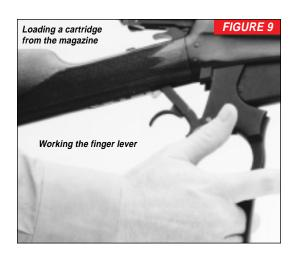
LOADING THE CHAMBER — The chamber may be loaded two ways:
