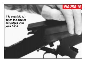
BEFORE UNLOADING, CHECK TO ASSURE THAT THE SAFETY (MANUAL HAMMER STOP) IS IN THE "ON" POSITION (SAFE) BY PULLING IT FULLY TO THE REAR UNTIL THE "S" JUST FORWARD OF THE SAFETY IS VISIBLE. KEEP YOUR FINGER AWAY FROM THE TRIGGER WHEN CYCLING THE ACTION.
